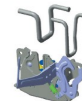
Hood safety mechanism with double striker
